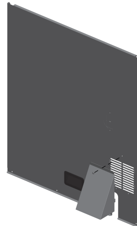
Figure 14. Vent hood installation
