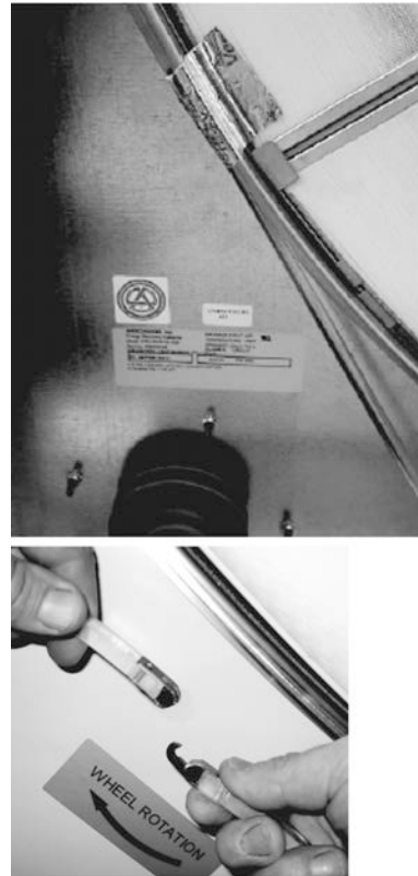
Figure 101. Link belt installation
