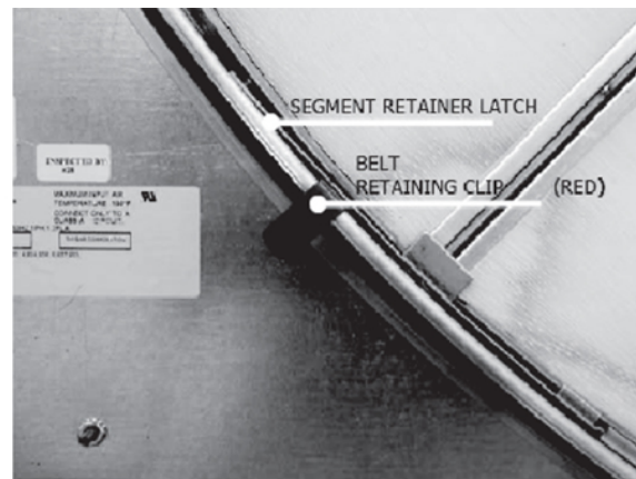
Figure 102. Retaining clip location
