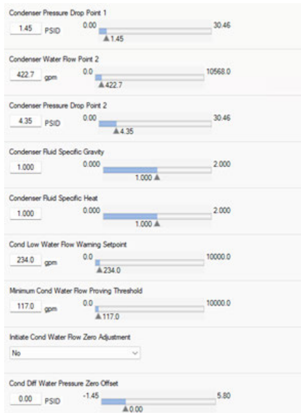
Figure 55. Settings for condenser water flow calibration
