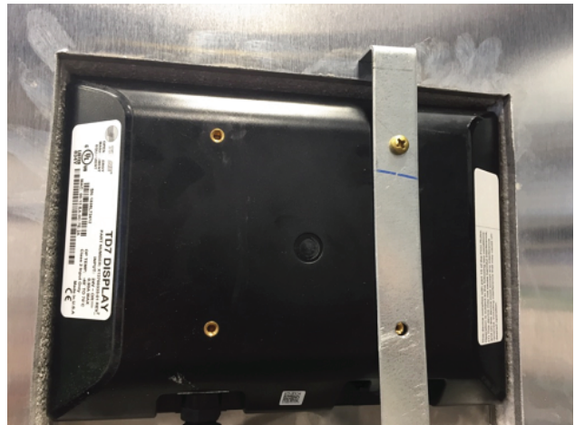
Figure 43. TD-7 Installation on back with brackets
