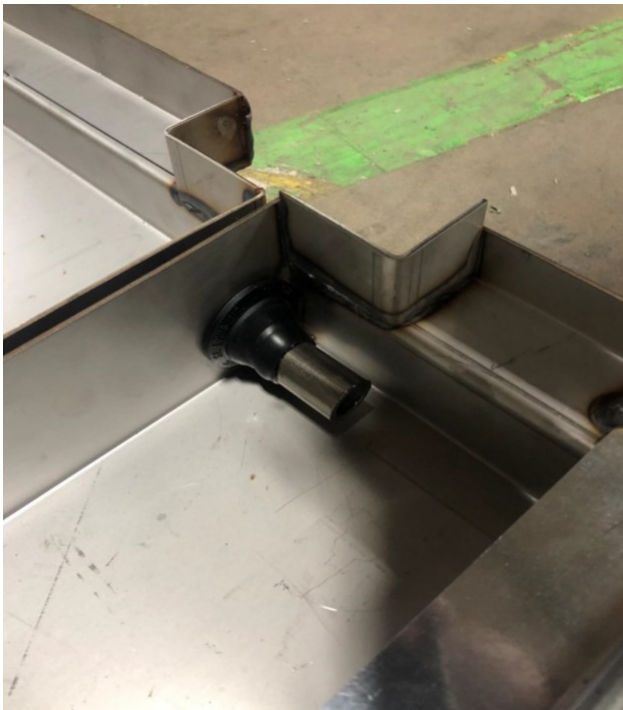
Figure 23. Joined drain pan installation
