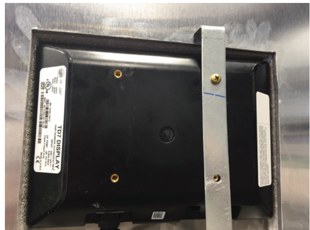
Figure 43. TD-7 Installation on back with brackets
