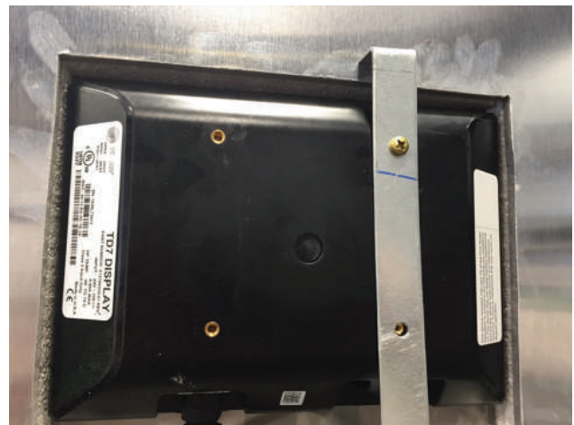
Figure 37. TD-7 Installation on back with brackets
