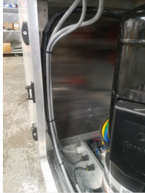
Figure 25. Compressor communication terminations
