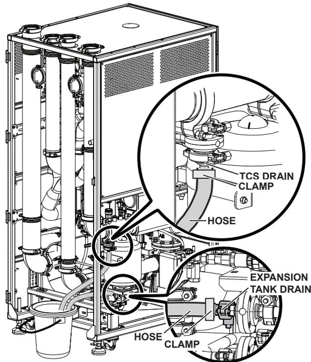
4. Connect one end of a hose to each of the TCS strainer drains, and route the other end of the hoses into the same container. Keep the other ends of the hoses above the liquid level to allow for air intake. Use a clamp to make sure the hose is installed securely.
