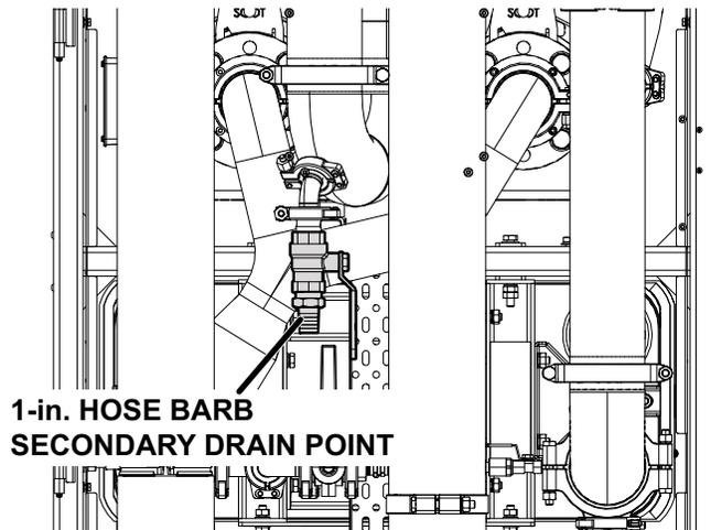
**Figure 36. 3-way valve / 2-way PICV TCS strainer drain point**
