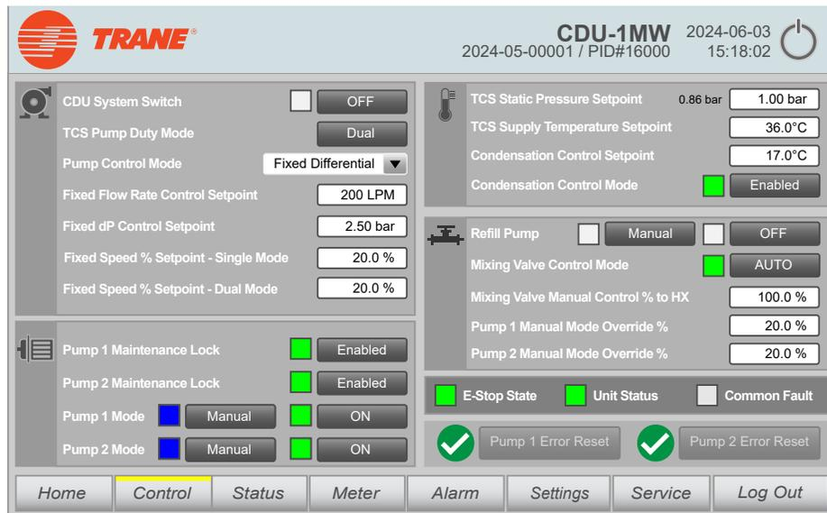
The corresponding CDU with a pump set to operate in **Manual** mode will be considered to be in a running state regardless of the command is from the Principal CDU.
