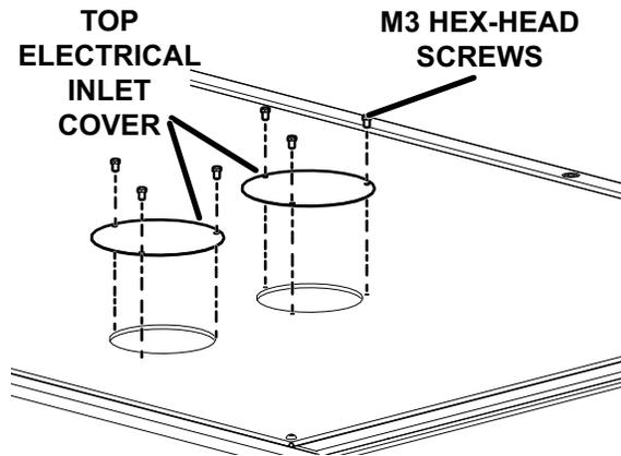
3. The top of the electrical panel has two holes with two blanking plugs used to install two PG29 cable glands. Remove the blanking plugs on top of the electrical panel, and remove the cable glands located at the bottom of the electrical panel.
