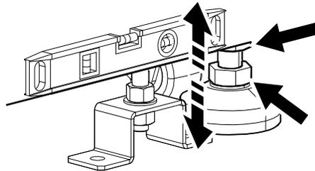
2. The unit may be secured to the floor, if required, with bolts suitable for the floor and the provided anchor bolt mounting brackets: two on the front and two on the rear.
