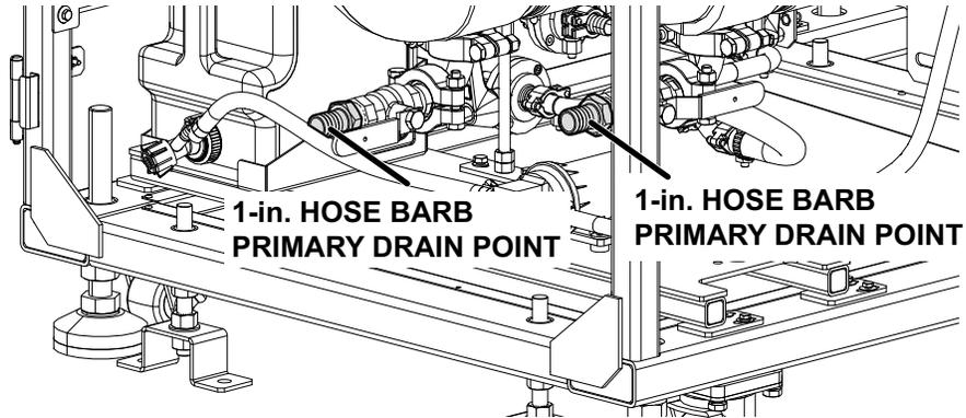
**Figure 32. 3-way valve rear (bottom piping)**
