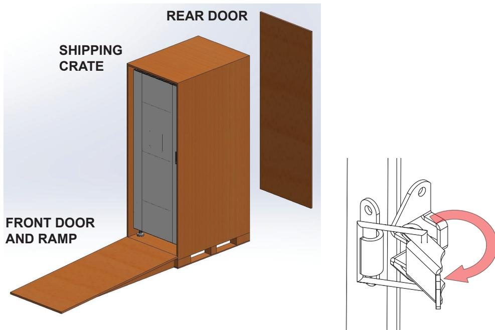
1. Open the butterfly locks securing the ramp in place and lower the ramp to the floor.
