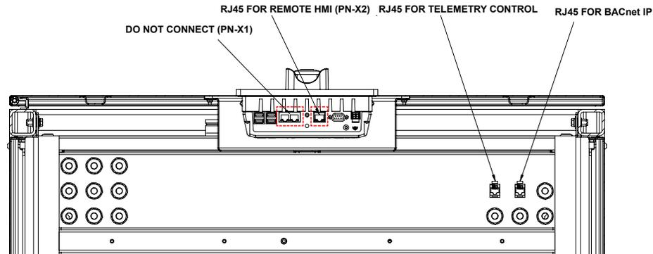
The RJ45 for remote HMI connection (PN-X2) is used for external communication. This is used for external communication via SmartClient (VNC), HMI web server. The IP address can be configured by DHCP or fixed IP to connect to an outside network. PN-X1 is the connection between the HMI and the PLC, and is used for internal communication only.
