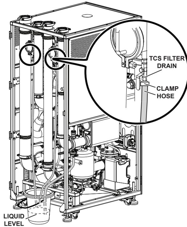
5. Open the valves to the TCS drain and expansion tank drain, and then open the TCS strainer drains.
