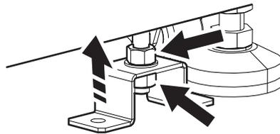
6. Use a 32-mm (M24) open-ended wrench to lift each leveling foot high enough so the unit can be rolled out of the shipping crate.
