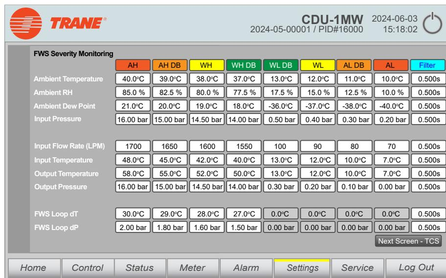
**Table 27. Severity Monitoring Threshold screen codes**
