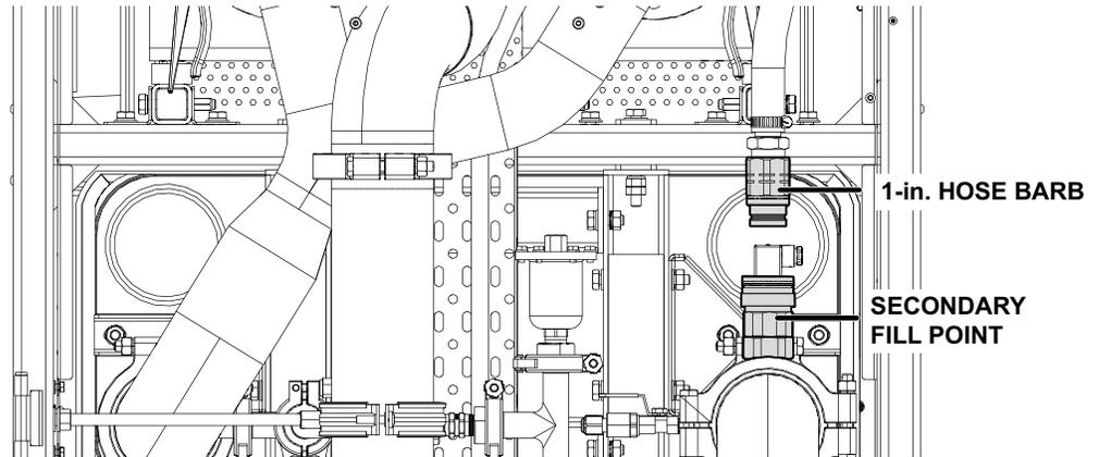
5. Connect the plug quick-connect to the receptacle quick-connect of the secondary fill point located on the TCS water circuit.
