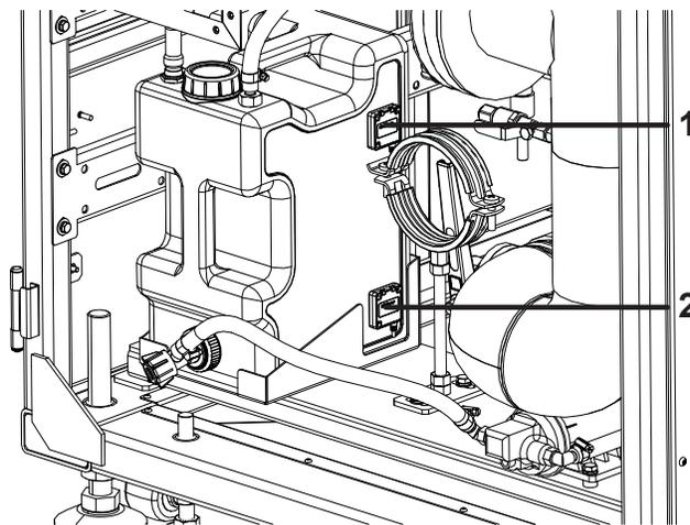
**Table 28. Automatic refill pump operation (3-way valve) description**
