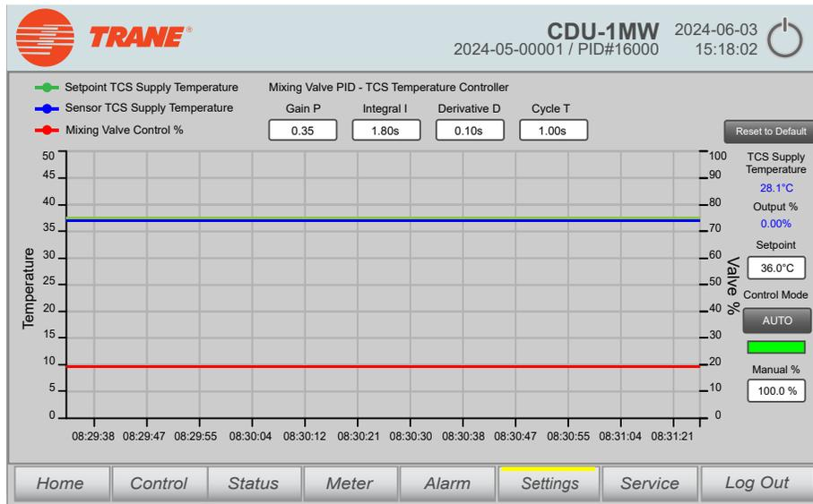
The left Y-axis measures temperature and is used with the Setpoint TCS Supply Temperature (green) line and the Sensor TCS Supply Temperature (blue) line. The right Y-axis measures the valve opening percentage and is used with the Mixing Valve Control % (red) line.
