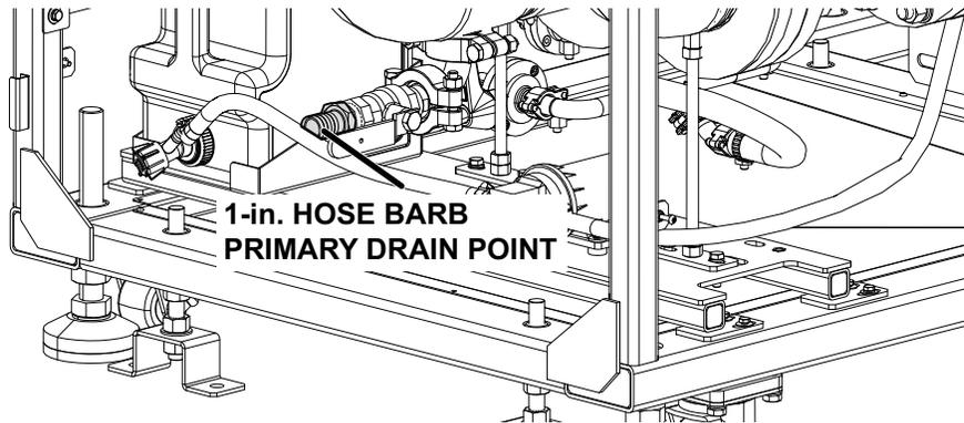
**Figure 34. 2-way PICV rear (bottom piping)**
