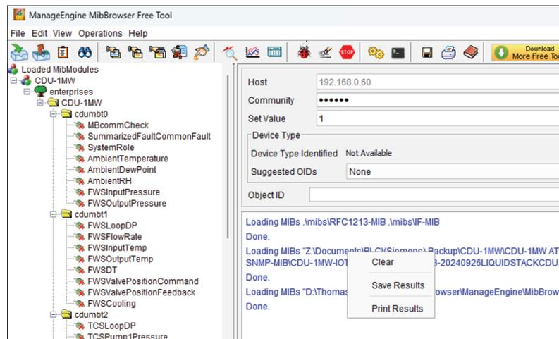
8. If the user selects any parameter on the left side, the description of the selected parameter is shown in the area near the bottom.
