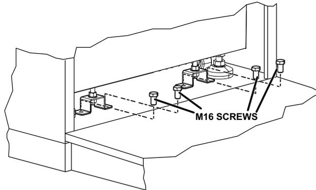
5. Use a 24-mm (M16) open-ended wrench to loosen the hex nuts and raise the anchor brackets so they do not interfere with movement of the unit. Re-tighten the hex nuts to secure the brackets in place.
