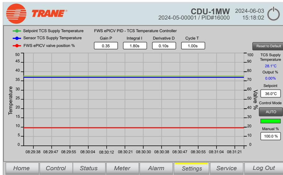
The left Y-axis measures temperature and is used with the Setpoint TCS Supply Temperature (green) line and the Sensor TCS Supply Temperature (blue) line. The right Y-axis measures the valve opening percentage and is used with the FWS Valve Control % (red) line.
