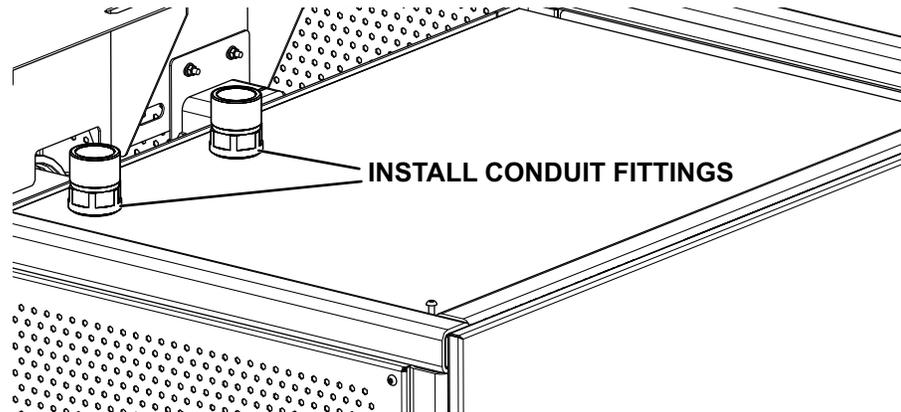
5. Insert the power cable through the cable gland located on top of the TCDU. Tighten the cable glands.
