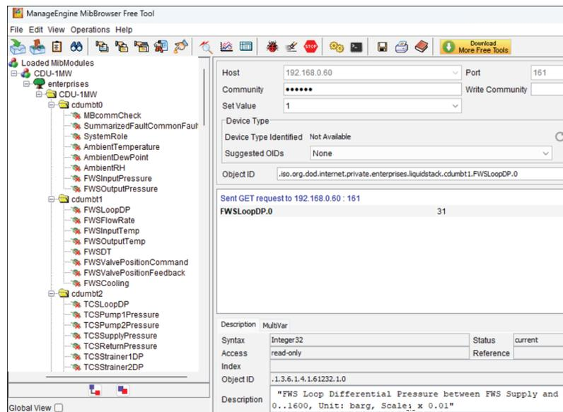
11. To retrieve all the values under the tree table, the user can right-click on **Trane** and select **SNMPWALK**. All the data values will then be listed out at the TCDU SNMP agent.
