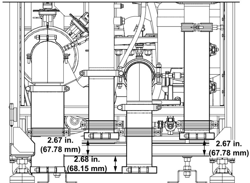
**Figure 19. Bottom piping access dimensions**
