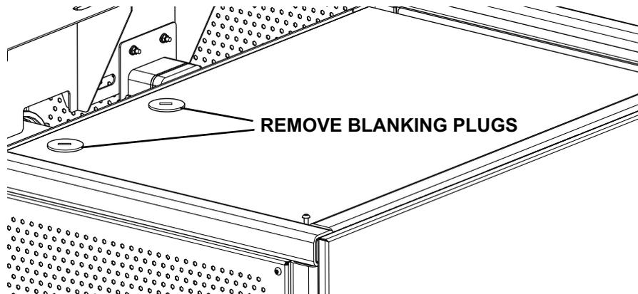
4. Install the cable glands in place of the blanking plugs on top of the electrical panel, and install the blanking plugs on the bottom where the cable glands were located. Alternatively, two PG29 conduit fittings (Field Supplied) could be used instead of the cable glands.
