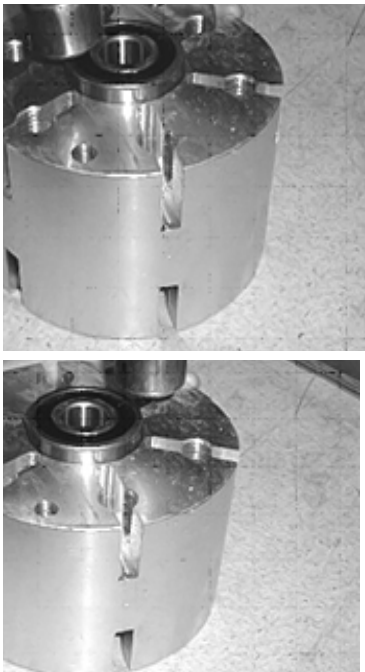
Figure 170. Tap outer race of new bearing, alternating sides
