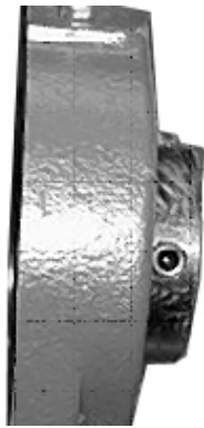
Figure 175. Loosen set screws
