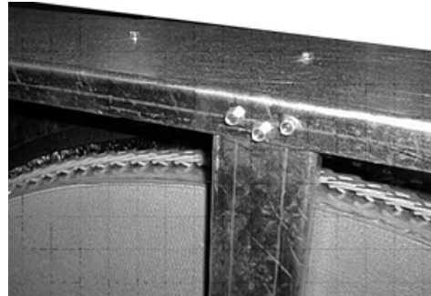
Figure 167. Remove post mounting screws
