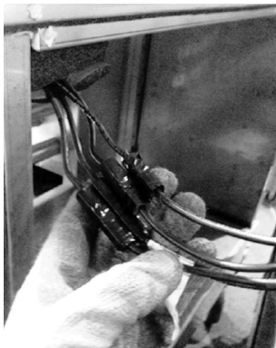
Figure 36. Horizontal section-to-section high voltage quick connects
