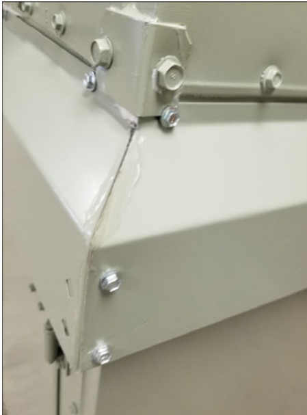
Figure 45. Stacked corner seam
