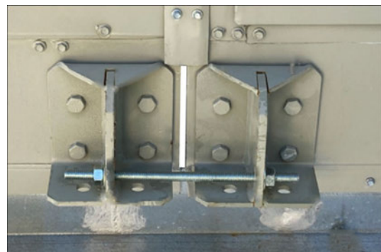
Figure 9. Shipping split seam – top view
