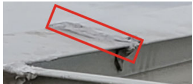
Figure 24. Two-piece wide roof strip caulk
