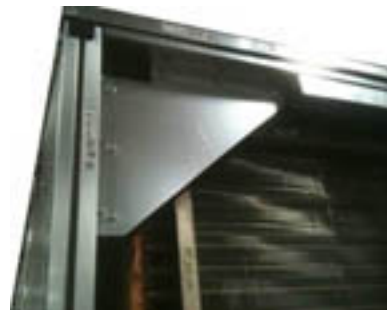
Figure 9. Shipping split seam – top view
