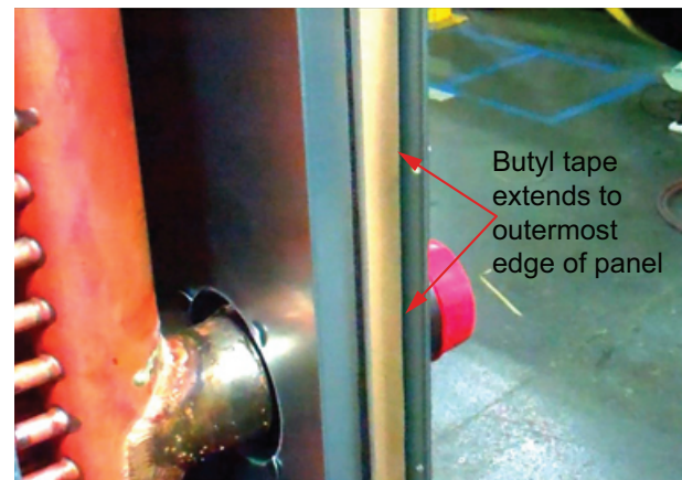
Figure 25. Install gasket to outermost edge of panel
