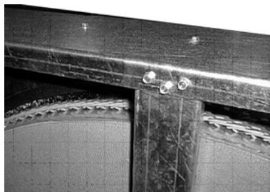
Figure 170. Remove post mounting screws
