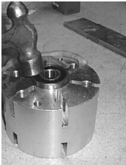
Figure 173. Tap outer race of new bearing, alternating sides
