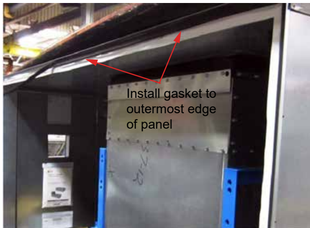
Figure 35. Install gasket to outermost edge of panel
