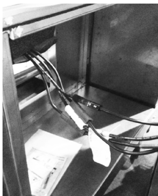
Figure 39. Horizontal section-to-section high voltage quick connects
