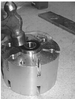
Figure 173. Tap outer race of new bearing, alternating sides
