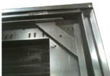
Figure 31. Coil structural gusset
