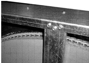
Figure 170. Remove post mounting screws
