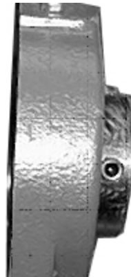
Figure 176. Loosen set screws
