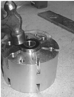
Figure 171. Tap outer race of new bearing, alternating sides
