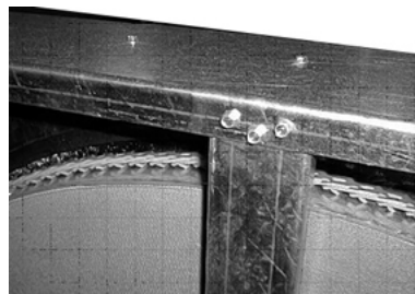
Figure 168. Remove post mounting screws
