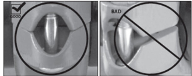
Figure 19. Metal-to-metal contact across the bolt pad section
