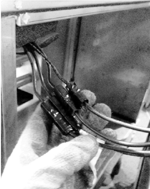
Figure 7. Section-to-section high voltage quick connects
