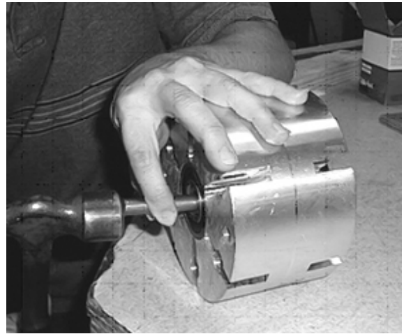
Figure 77. Remove old bearing by tapping from the back. Gently tap around the race. Repeat on opposite side.
