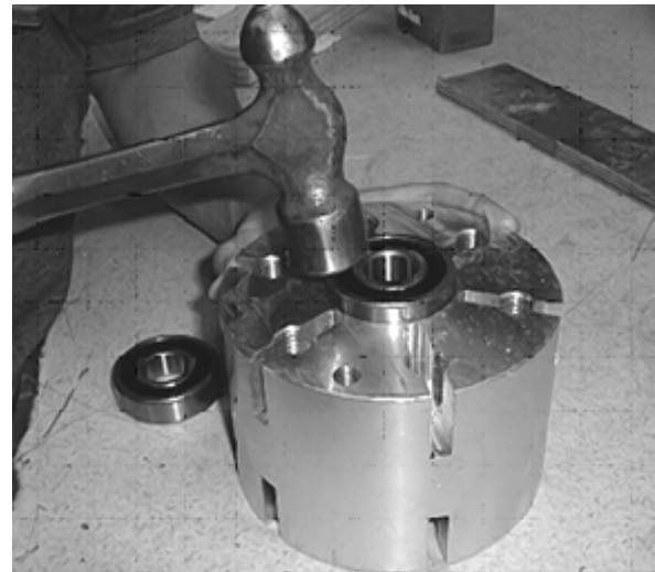
Figure 78. Tap outer race of new bearing, alternating sides
