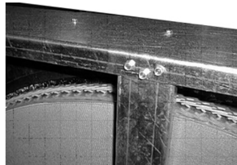
Figure 73. Remove post mounting screws
