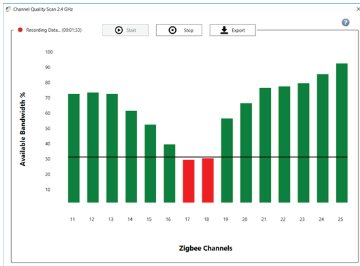
Figure 77. Real-Time Scan screen showing channels 17 and 18 with heavy traffic that will not support Air-Fi communication
