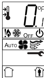
Figure 41. Wrench symbol signifying configuration mode
