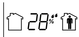
Figure 30. Display screen of a WCS with an RH sensor module
