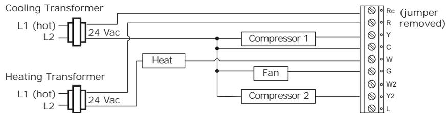
**Figure 19. 3H/2C Non-Programmable Thermostat, 2H/2C, Heat Pump Without Auxiliary Heat (Option 8)**
