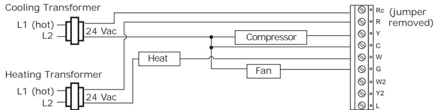
**Figure 12. 3H/2C Non-Programmable Thermostat, 1H/1C, Heat Pump Without Auxiliary heat (Option 1)**
