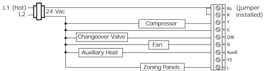
**Figure 17. 3H/2C Non-Programmable Thermostat, 2H/1C, Conventional (Option 6)**
