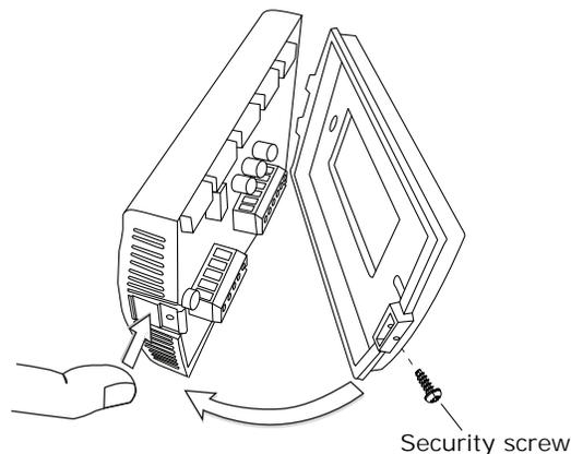
2. Remove the cover by firmly pressing the thumb tab at the bottom of the cover and pulling the cover away from the back plate.
