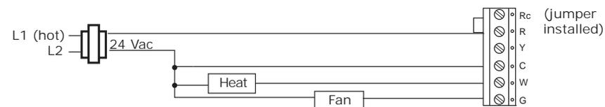
**Figure 10. 1H/1C Thermostat, 1C Only, Conventional (option 4)**
