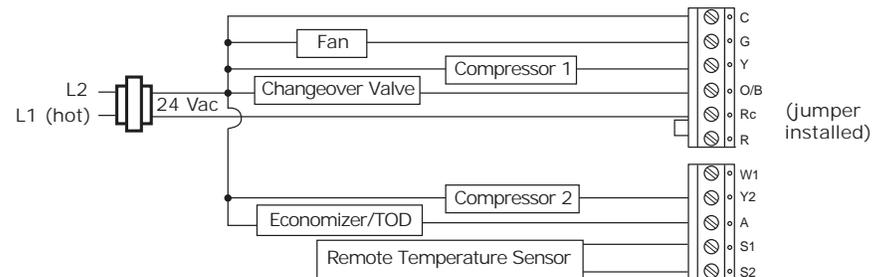
**Figure 31. Programmable Thermostat, 3H/2C, Heat Pump With Auxiliary Heat (Option 11)**
