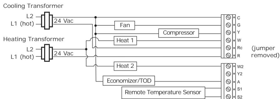
**Figure 29. Programmable Thermostat, 1H/2C, Conventional (Option 9)**
