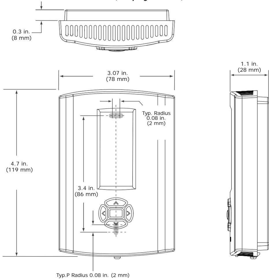
**Note:** Drawing not to scale. Dimensions within  $\pm 0.02$  in. ( $\pm 0.5$  mm)
