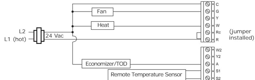
**Figure 25. Programmable Thermostat, 1C, Conventional (Option 5)**
