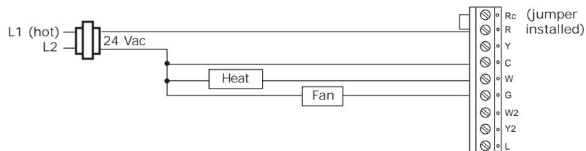
**Figure 15. 3H/2C Non-Programmable Thermostat, 1C, Conventional (Option 4)**
