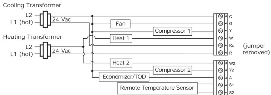
**Figure 28. Programmable Thermostat, 2H/1C, Conventional (Option 8)**
