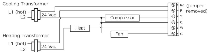
**Figure 7. 1H/1C Thermostat, 1H/1C Heat Pump Without Auxiliary Heat (Option 1)**
