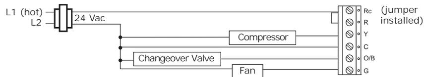
**Figure 8. 1H/1C Thermostat, 1H Only, Conventional Without Fan (Option 2)**
