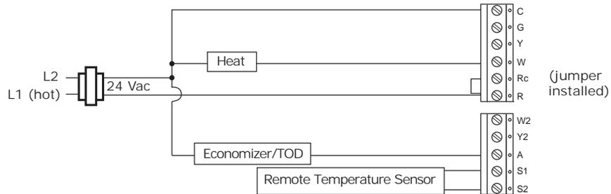
**Figure 24. Programmable Thermostat, 1H, Conventional With Fan (Option 4)**
