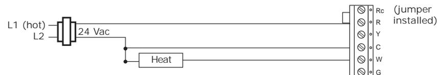
**Figure 9. 1H/1C Thermostat, 1H Only, Conventional With Fan (option 3)**
