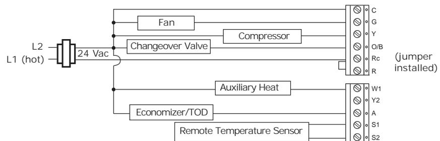
**Figure 27. Programmable Thermostat, 2H/2C, Conventional (Option 7)**
