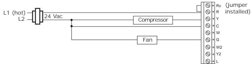
**Figure 16. 3H/2C Non-Programmable Thermostat, 2H/1C, Heat Pump With Auxiliary Heat (Option 5)**
