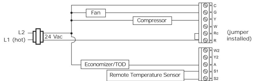
**Figure 26. Programmable Thermostat, 2H/1C, Heat Pump With Auxiliary Heat (Option 6)**
