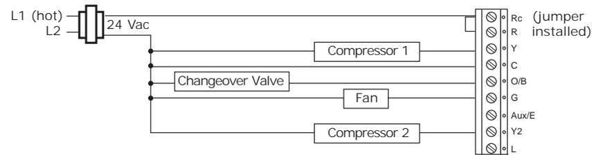
**Figure 20. 3H/2C Non-Programmable Thermostat, 3H/2C, Heat Pump With Auxiliary Heat (Option 9)**
