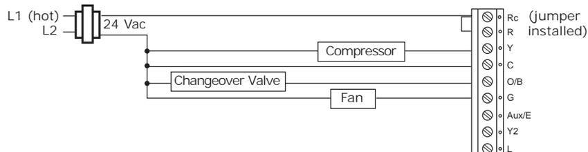
**Figure 13. 3H/2C Non-Programmable Thermostat, 1H Only, Conventional Without Fan (Option 2)**
