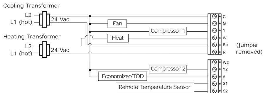
**Figure 30. Programmable Thermostat, 2H/2C, Heat Pump Without Auxiliary Heat (Option 10)**
