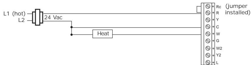
**Figure 14. 3H/2C Non-Programmable Thermostat, 1H, Conventional With Fan (Option 3)**
