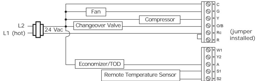
**Figure 23. Programmable Thermostat, 1H Only, Conventional Without Fan (Option 3)**
