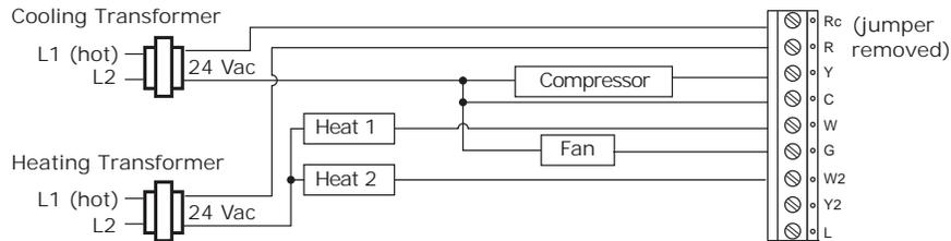
**Figure 18. 3H/2C Non-Programmable Thermostat, 1H/2C, Conventional (Option 7)**
