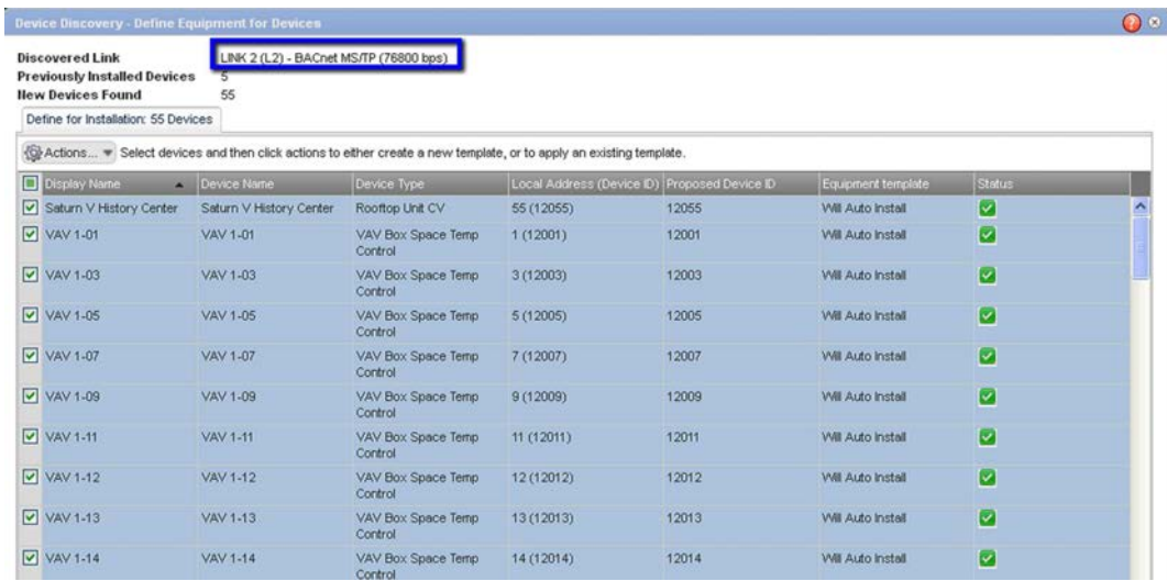
Figure 74. BACnet devices: will auto install
