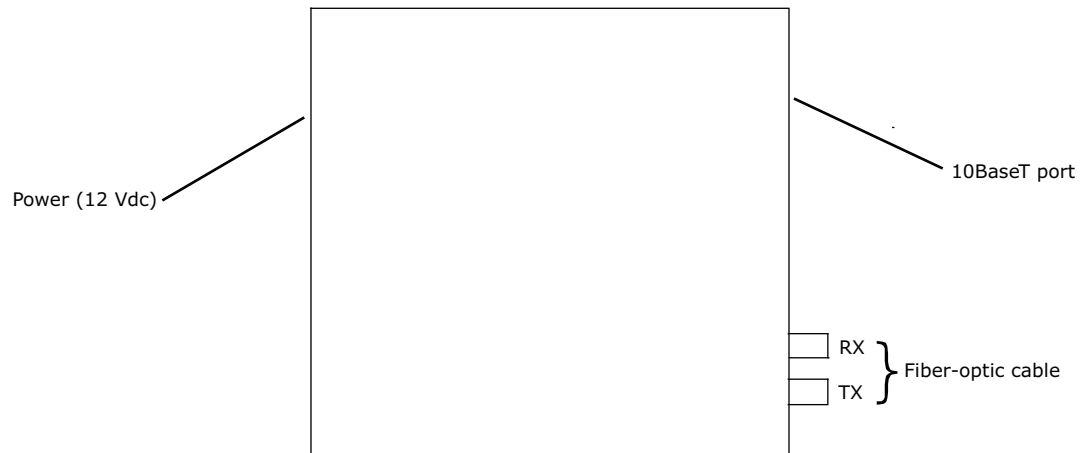
Figure 57. Fiber-optic media converter for 10BaseT wire (connect Air Int. W4869)
