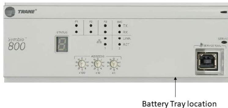
Figure 3. Symbio 800 battery tray location
