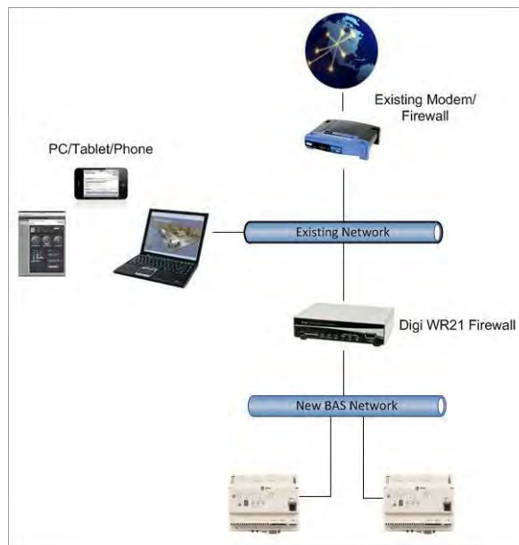
Figure 2. Customer network after installation of Digi WR21Transport firewall
