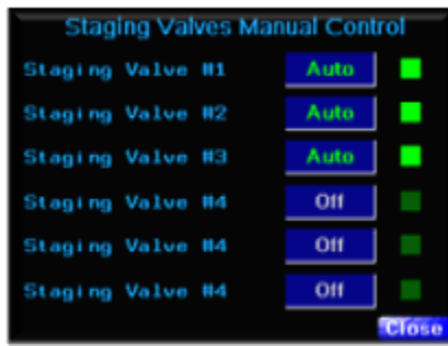
Figure 27. Staging valves control screen
