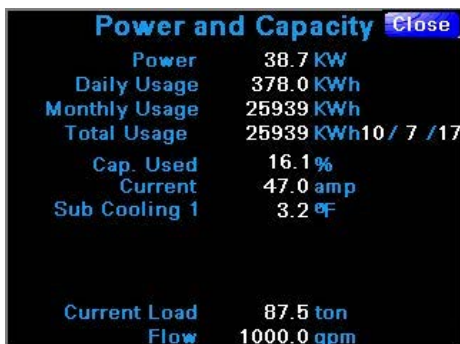
Figure 19. Power and capacity control screen
