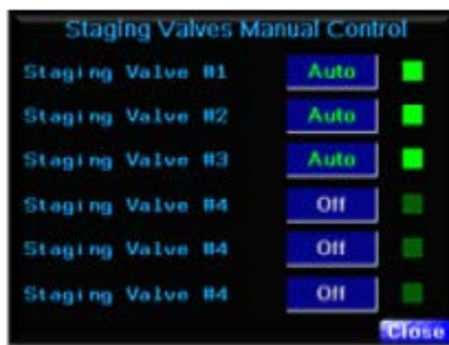
Figure 28. Staging valves control screen
