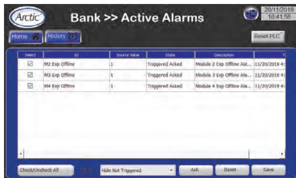
Figure 16. Active alarms for the chiller
