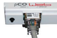
BACnet IP, BACnet Ethernet, HTTP, SNMP, and Modbus IP
